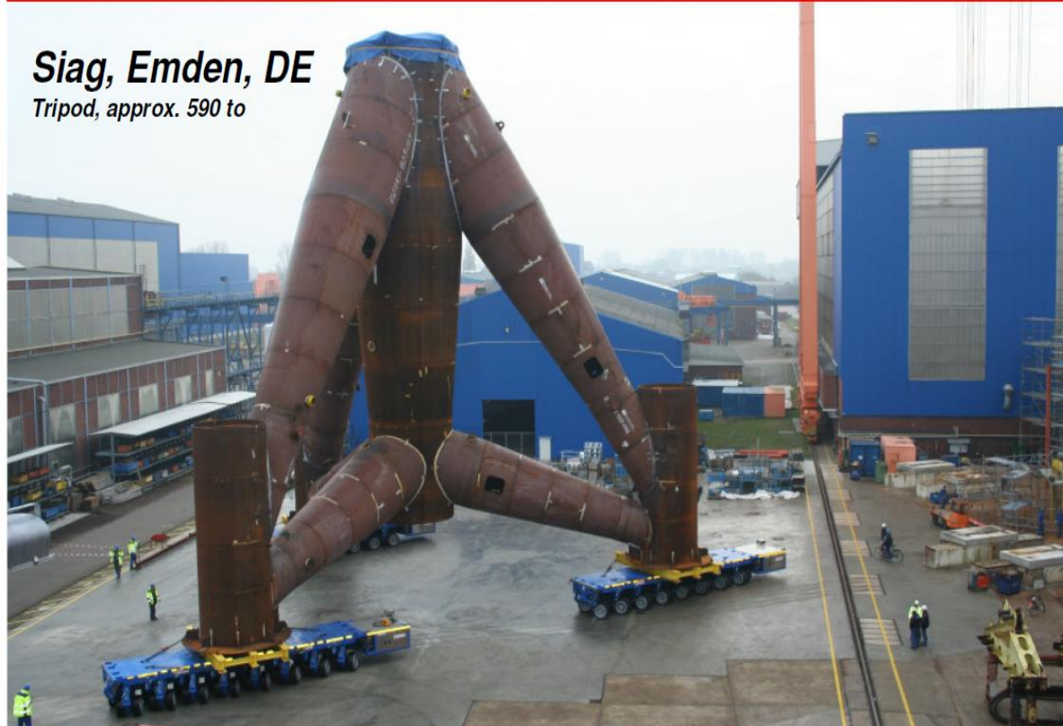
Figure 7: Tripod base on SPMT vehicles.
