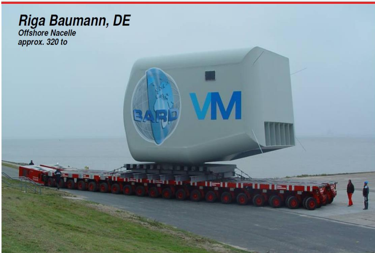
Figure 9: Nacelle on SPMT
