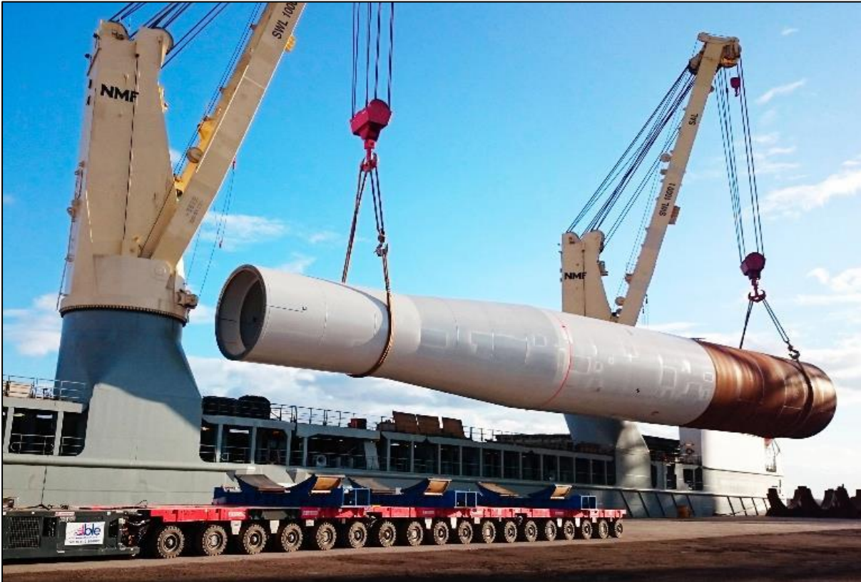
Figure 4: A Monopile (c. 1,000T) being unloaded onto a SPMT at Able Seaton Port
